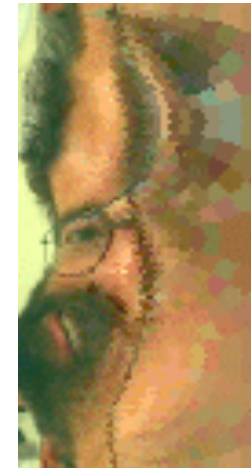
Transformation of log-polar image into a uniform, rectangular pixel tessellation [G. Sandini]
