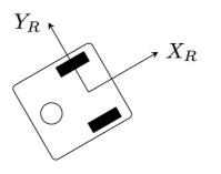
The motion of the robot in the local robot frame of reference R due to the rotation of the wheels is given by:
