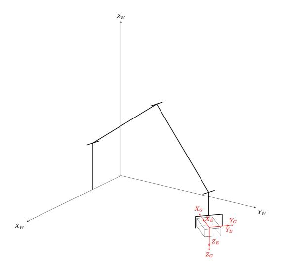
... the end-effector pose aligned with the object grasp pose
