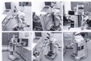
Fig. 1. Different object grasps selected by the generative model based on the object, task, and context.
