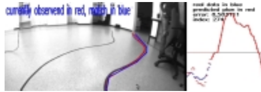
Fig. 2. Example of the planner operating mode. The observed street is compared to the database entries and the assigned steering sequence of the best match is depicted on the right.
