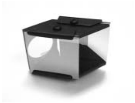
Figure 4. Prototype single sensor stereo device.
