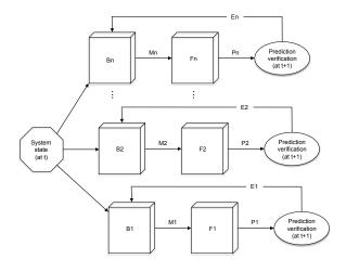
Fig. 3. The HAMMER architecture, showing multiple inverse models (B1 to Bn) taking as input the current system state, which includes a desired goal, suggesting motor commands (M1 to Mn), with which the corresponding forward models (F1 to Fn) form predictions of the system's next state (P1 to Pn). These predictions are verified at the next time state, resulting in a set of error signals (E1 to En). Redrawn from [27]. See also [28] for an alternative rendering of the HAMMER architecture.
