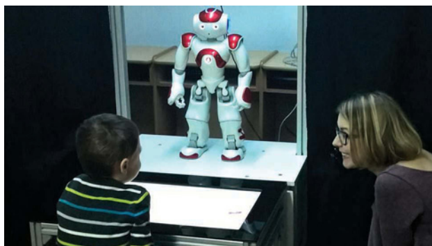
Figure 8. The intervention platform used in DREAM. A child sits in front of a robot and an interactive screen.
