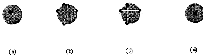
Fig. 9. Given a point within the blob, two line scans can be used to calculate a better estimate of the centroid.
