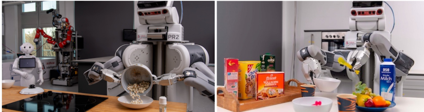
A PR2 robot pours popcorn from a saucepan (left) and sets a table (right) during demonstrations of cognitively-enabled robot manipulation using CRAM. Image courtesy of the Everyday Activity Science and Engineering (EASE) interdisciplinary research center at the University of Bremen, Germany.
